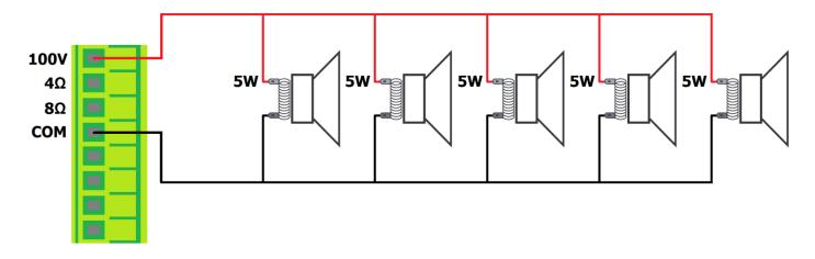
A 100V line speaker system can comprise of many speakers connected together. The determining factor for how many speakers can be used on a single amplifier is the power rating. For most purposes, it is advised to connect as many speakers as needed with a combined wattage of no more than 80% of the amplifier's output power rating (in the case of the PA-6120MX, this is 30W per zone output)
